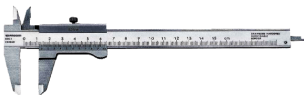
Figure : A vernier scale ; used to measure external and internal diameters of an object
