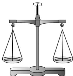
Figure : A beam balance ; used to measure mass
